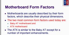
• Most new systems come with the ATX motherboard form factor.
